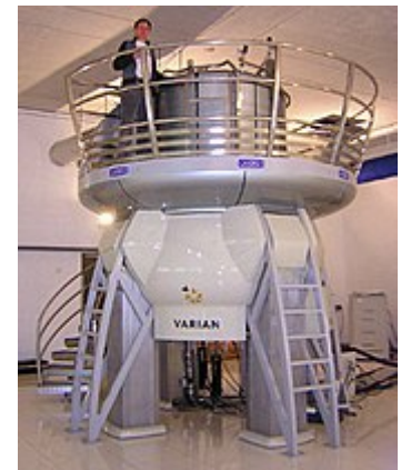
NMR Magnet at HWB-NMR, Birmingham, UK. In its strong 21.2-tesla field, the proton resonance is at 900 MHz.
